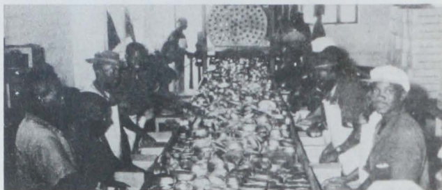
Fig. 8 - Conveyor and labeling machine in a South-West Africa pilchard cannery.
