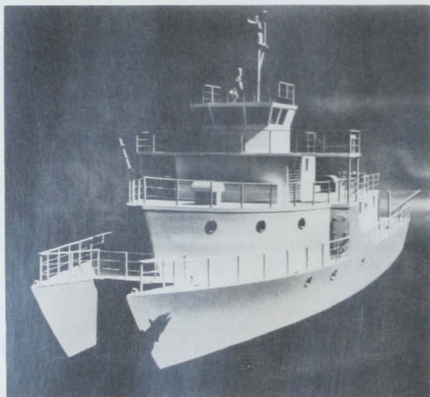
An artist's conception of the large twin-hulled aluminum catamaran, presently under construction, to be used for oceanographic research by Johns Hopkins University.
