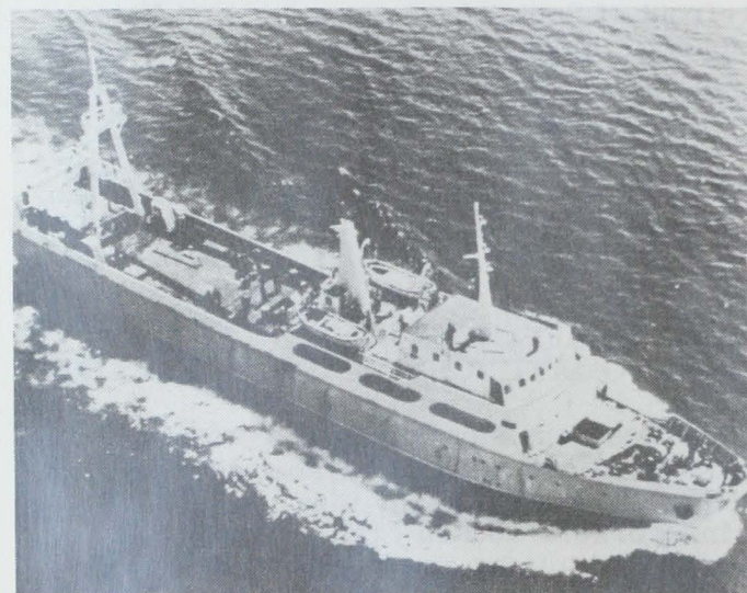
Fig. 3 - Freezer stern trawler built in 1964 designed for fishing shellfish and finfish. It is 929 gross registered tons.
