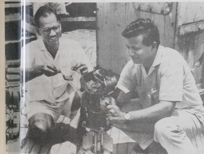
Fig. 1 - Two scientists from India, working guests, remove a sea floor sediment sample from a LaFond-Dietz bottom snapper.
