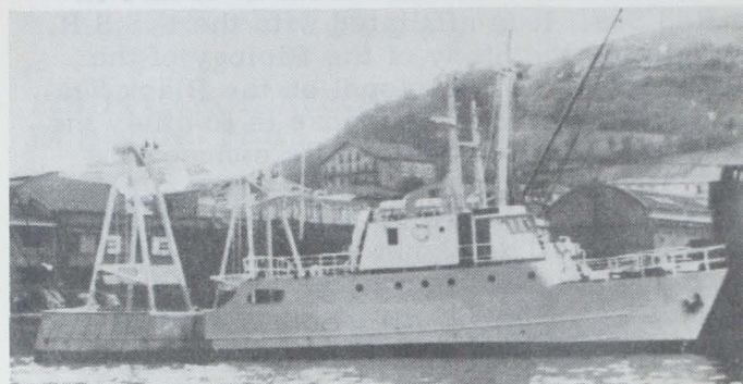
Fig. 2 - Freezer stern trawler built in 1965 for fishing shellfish. It is 158 gross registered tons.
