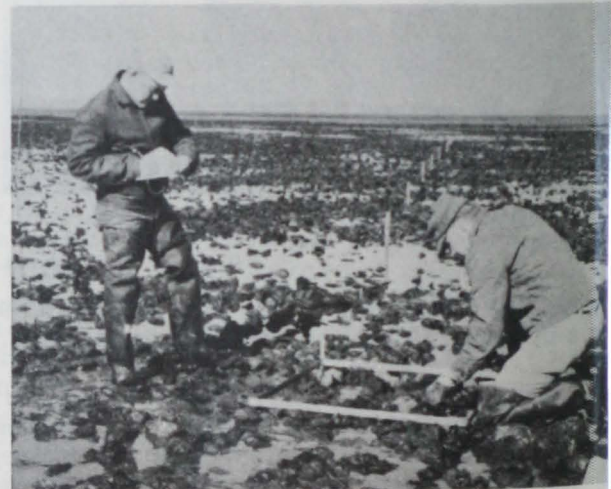
Fig. 6 - The square-yard sampler used for making a systematic count of live and dead oysters, amount of shell, and number of clusters. The line of cedar stakes indicates locations to be surveyed. (Photo by C. C. Larsen)
