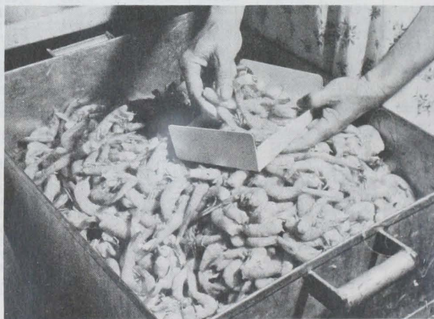
Fig. 1 - Packing heads-off fresh shrimp in consumer packages for freezing in a Florida plant.
