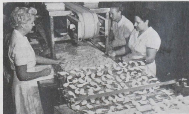
Fig. 2 - Breaching peeled and deveined shrimp at a Tampa, Fla., shrimp-processing plant. This method of processing shrimp for the convenience of the consumer has increased in importance in recent years.
