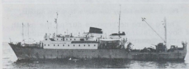
Fig. 1 - Large Soviet factory stern trawler of the "Tropik" class in the North Atlantic.
