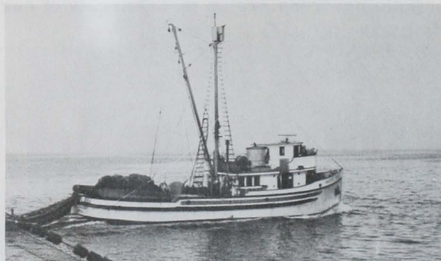
Fig. 2 - The 80-foot seiner Pacific Pride . The seine used is 250 fathoms long and seven 200-mesh strips deep. The mesh size is 1⅜" stretched. All nylon web is used.
