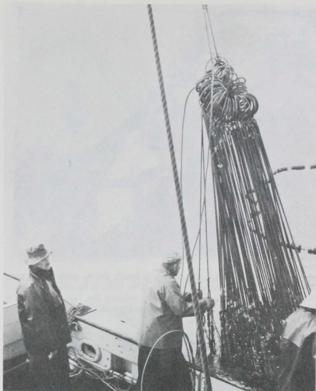
Fig. - 6 After the net is pursed, trapping the fish, the purse rings are brought aboard in preparation for hauling the seine aboard.
