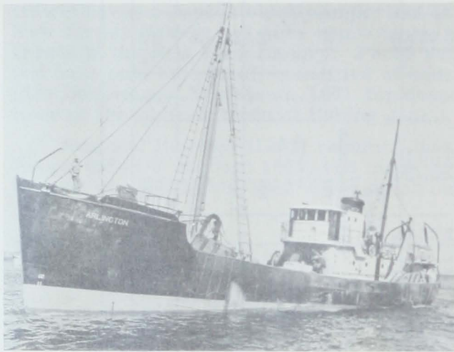
Fig. 8 - A Boston large steel otter trawler.
