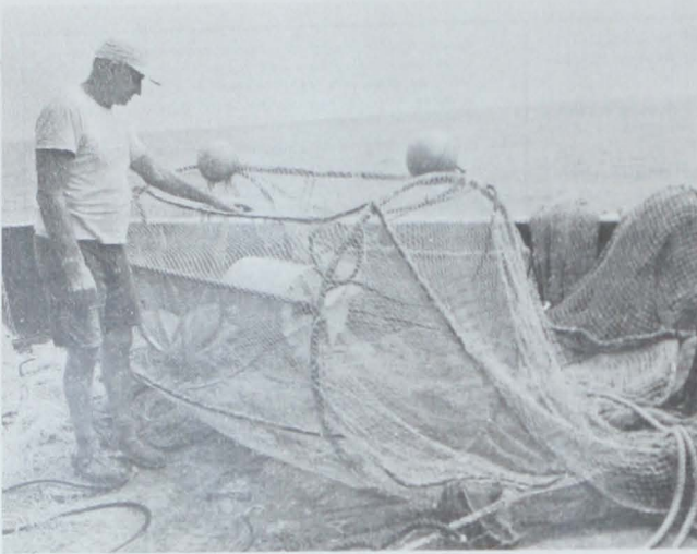
Housing of underwater movie camera attached to its frame in the mouth of a shrimp trawl. Used by the M/V Oregon for motion picture photography of both trawl performance and shrimp reaction behavior.
