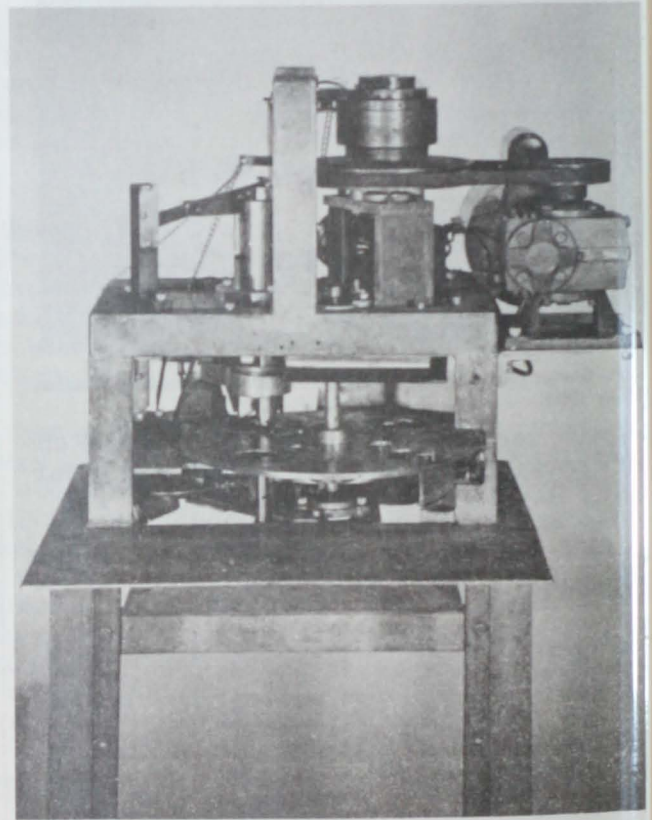
A semiautomatic machine that cleans and debacks whole cooked blue crabs.
