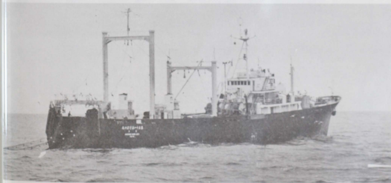
Fig. 1 - Trawl being hauled up the stern ramp of a 260-foot Japanese factory trawler in the eastern Bering Sea. The Japanese are rapidly adding to their fleets more of these highly capable ships which catch and process fish without need of accompanying factoryships.
