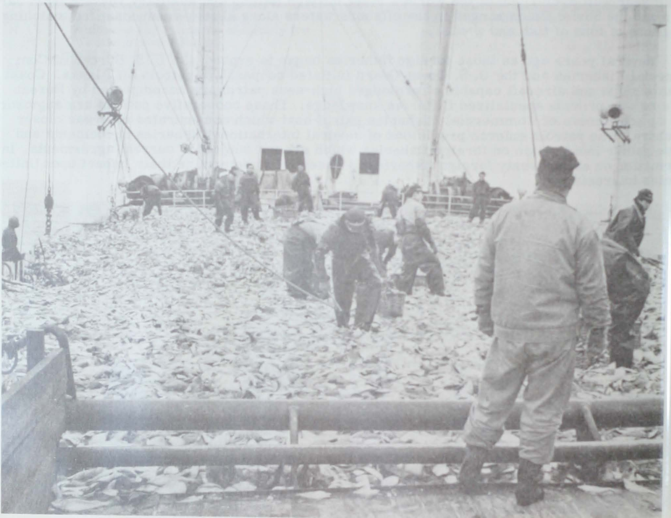
Fig. 2 - The deck of a Japanese factoryship is covered to a depth of several feet with flounder and sole caught in the eastern Bering Sea near Bristol Bay. Fleets of trawlers deliver their catches to the factoryship, where the fish are reduced to meal and oil within a few hours. Workers selecting larger fish which are frozen for human consumption wear snowshoe-like boards on their feet to keep them from sinking into the mass of fish.
