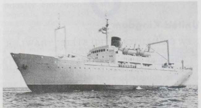
Freezer-trawler M/S Golfstrim--a refrigerator vessel that can also be used as a trawler.
