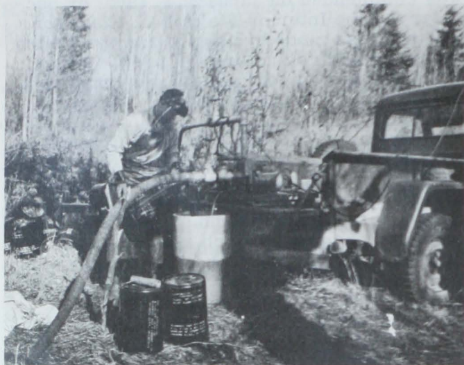
Fig. 2 - Feeder mechanism that maintains critical level of selective toxicants in Great Lakes streams infested with sea lampreys. The chemicals introduced in the streams selectively kill the young lamprey.
