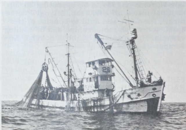
A Korean mackerel seiner equipped with a power block for hauling in the seine net.
