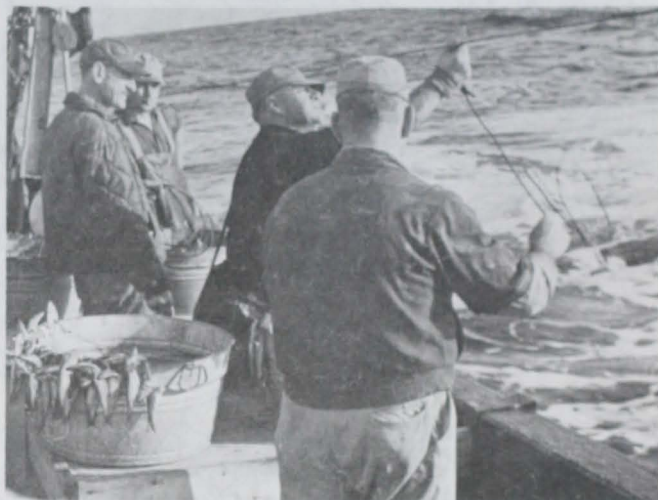
Fig. 1 - Set-out of long-line gear from powered reel during Delaware cruise 64-10. Note A-K type snap (with branchline) being applied to 20-fathom mainline section.
