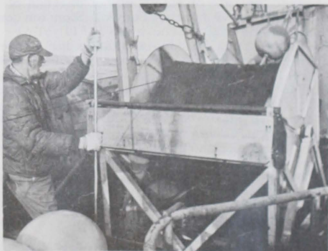
Fig. 2 - Powered long-line reel hauled long-line gear during Delaware cruise 64-10. Hydraulic motor and reducer are at lower left corner of frame. Manual level-winding was required after breakdown of mechanical level-wind device.
