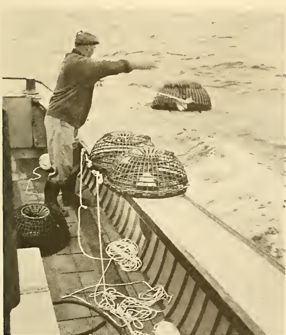
Fig. 4 - Lobster fisherman throws an "igloo" trap overboard. Weighing 25 pounds, the plastic traps are lighter than conventional traps which can weigh up to 100 pounds when water soaked. The new traps weigh about the same as the wooden traps on the bottom, 19 pounds, because of their lower buoyancy. The iron ring at the base distributes the weight around the circumference of the "igloo" trap giving it stability on the bottom.
