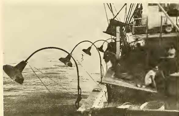
Fig. 2 - Philippine purse-seine vessel ready to begin night-light fishing in Sulu Sea. Note metal lamps set over the side to attract fish. Often it is midnight before enough fish are attracted to justify setting the purse-seine net.
