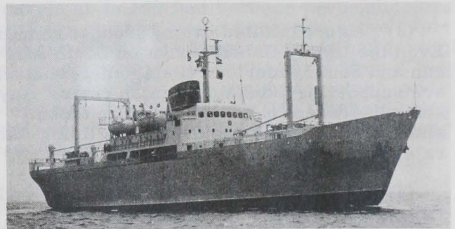
The 2,570-ton freezer-trawler M/S Gletcher , a refrigerator vessel that can also be used as a trawler.
