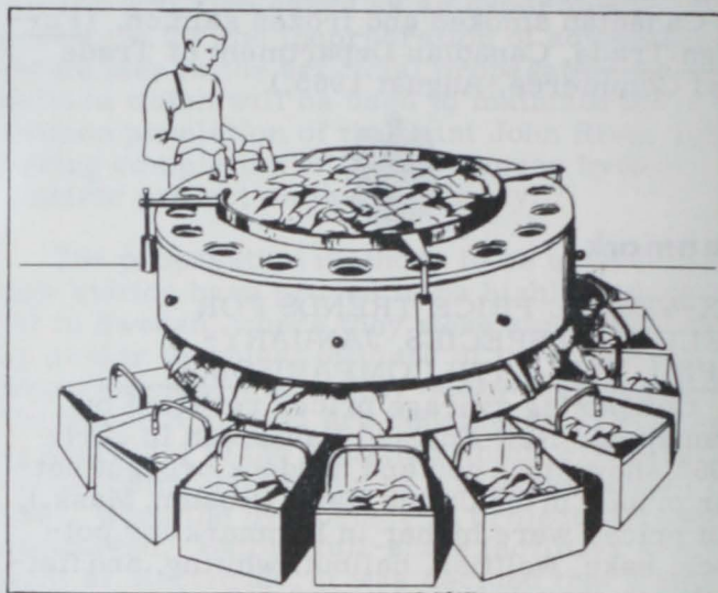
A fillet-grading machine used in a Danish fish-filleting plant.
