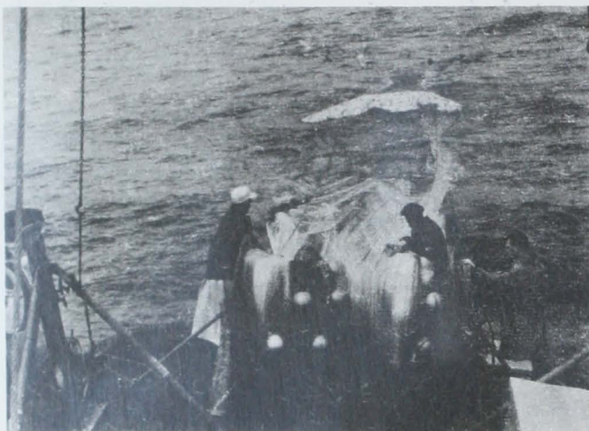
Fig. 3 - Incremental hang-in along corner riblines is illustrated in photograph of the "Cobb" pelagic trawl being reeled aboard the St. Michael. This catch is approximately 42,000 pounds of Pacific hake taken in a 60-minute tow. The same catch is also shown alongside vessel in fig. 12.
