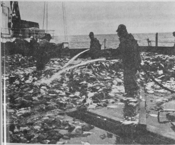
Fig. 4 - Washing silt and dirt from net loads of trawl-caught fish on the main deck of a typical Japanese factoryship.
