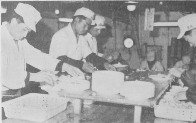
Fig. 5 - Sorting and weighing king crab meat prior to freezing aboard a Japanese crab factoryship.
