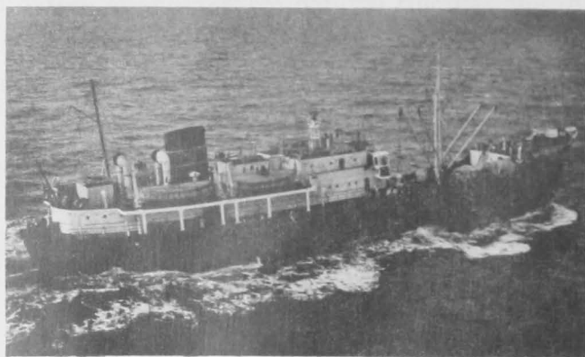
Fig. 1 - One type of Soviet factoryship operating in the North Pacific and Bering Sea. Length over-all about 150 feet with a speed of 10-12 knots.
