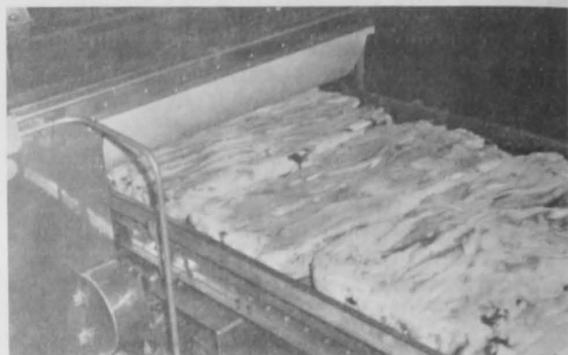
Fig. 3 - Frozen blocks of whole fish entering thawing unit.
