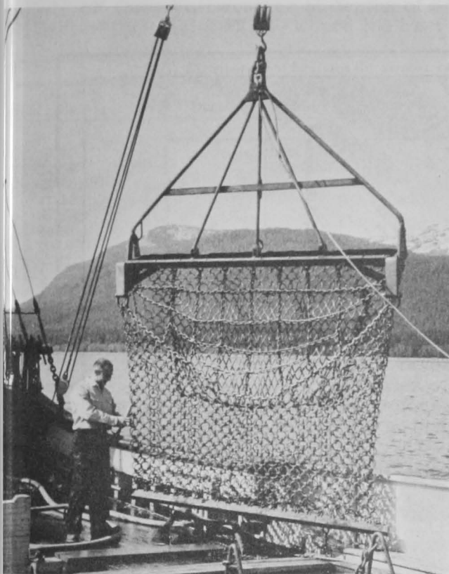
Fig. 2A - Eight-foot scallop dredge similar to the equipment used in the scallop fishery of the Northwest Atlantic. Note the rock chains ahead of the sweep chain.
