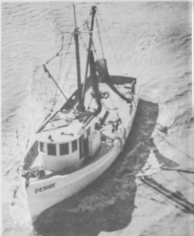
A typical Louisiana offshore trawler of about 60 ft. over-all length and 16 net tons.
