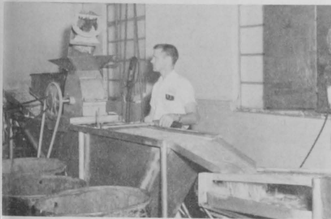
Fig. 28 - This is a patented crab-picking machine sometimes known as a claw cracker. The screw-conveyor elevates the claws to the hopper of a special type of hammermill. The broken pieces fall into a separation tank from which the meat floats off to an inspection-conveyor belt at the left. A U.S. Department of the Interior fishery inspector is observing the operation.
