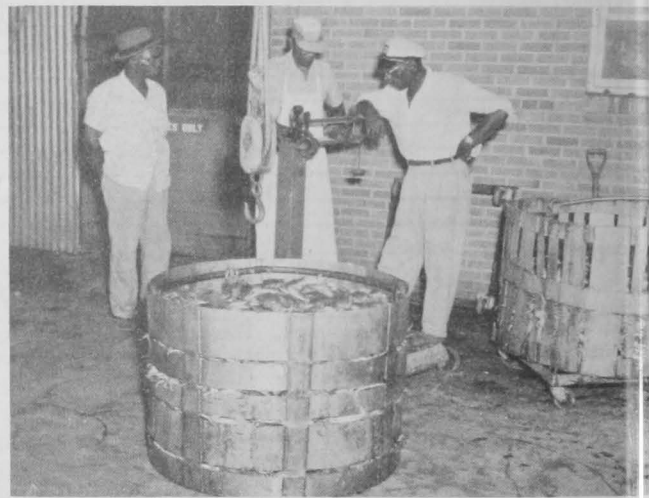
Fig. 10 - This plant uses circular retort baskets in which the crabs are cooked. Each basket holds 300 to 400 pounds of crabs.
