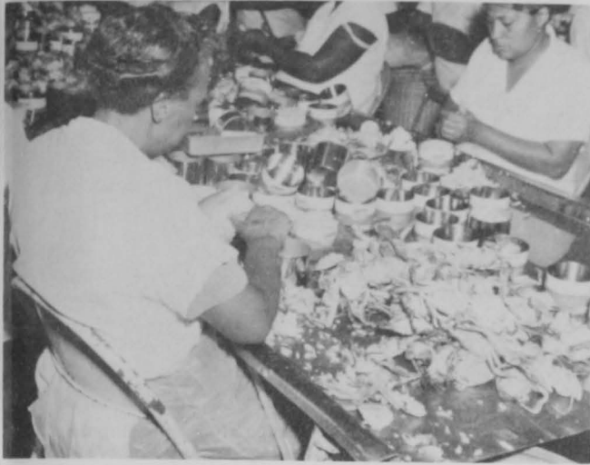
Fig. 26 - The cartilage is cut and the meat picked out with a special knife.
