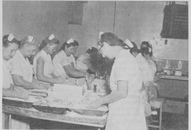
Fig. 39 - The frozen shell-with-deviled-crab-mix is hand dipped in batter and breading and then is packed into boxes.
