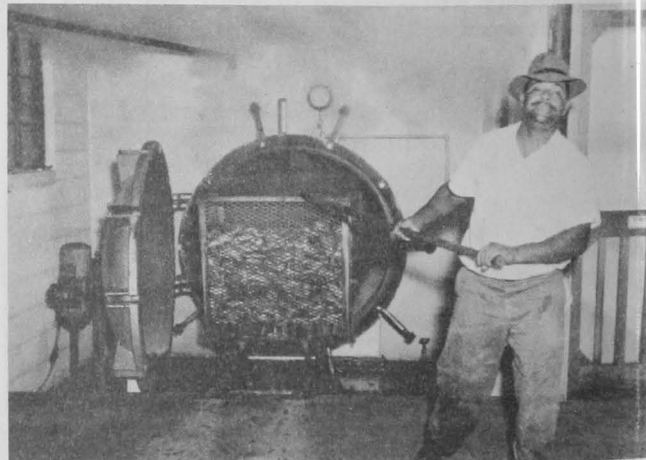
Fig. 12 - Other plants use horizontal pressure cookers. This cooker holds 4 of the wheeled steel mesh carts.
