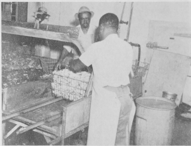
Fig. 22 - Here the debacked "cores" are washed by water sprays in an elevated flume and are transported to a basket at the end of the debacking table.
