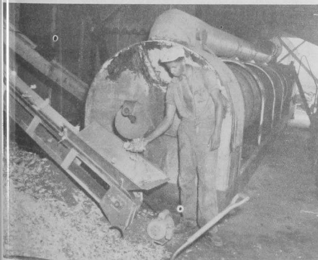
Fig. 17 - At the discharge end of another dryer, a worker is checking the scrap to determine if it is sufficiently dry for grinding.
