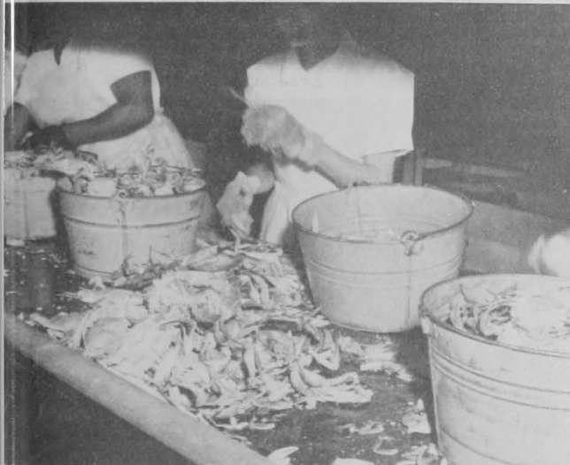
Fig. 15 - These workers are debacking or "bobbing" crabs. Claws are removed at the same time, as they are picked separately. The shell and viscera are discarded. Since the yield of crab meat amounts to only 12 to 15 percent of the weight of whole crab, disposing of the waste is a problem.
