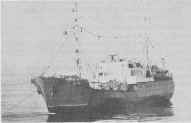
Fig. 4 - Trawler of Okean class. Has refrigerated holds. Vessel uses conventional side trawl, and is also equipped for gill-netting.
