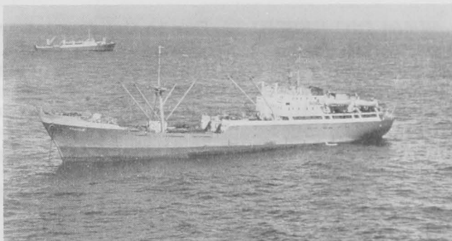
Fig. 8 - Refrigerator transport of the Tavriia class. On board are facilities for quick-freezing and storing fish brought to the vessel by a fleet of fishing craft.
