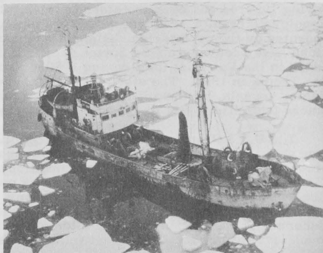
Fig. 3 - Trawler of SRT class. Vessel has no refrigeration equipment.
