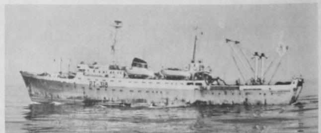
Fig. 5 - Stern trawler of the Maiakovskii class. Known also as a BMRT , the vessel is a completely integrated fishing and processing factoryship with freezing, canning, and reduction equipment.
