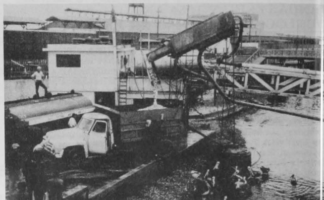
Fig. 3 - The fish are being pumped from the boat to awaiting truck.
