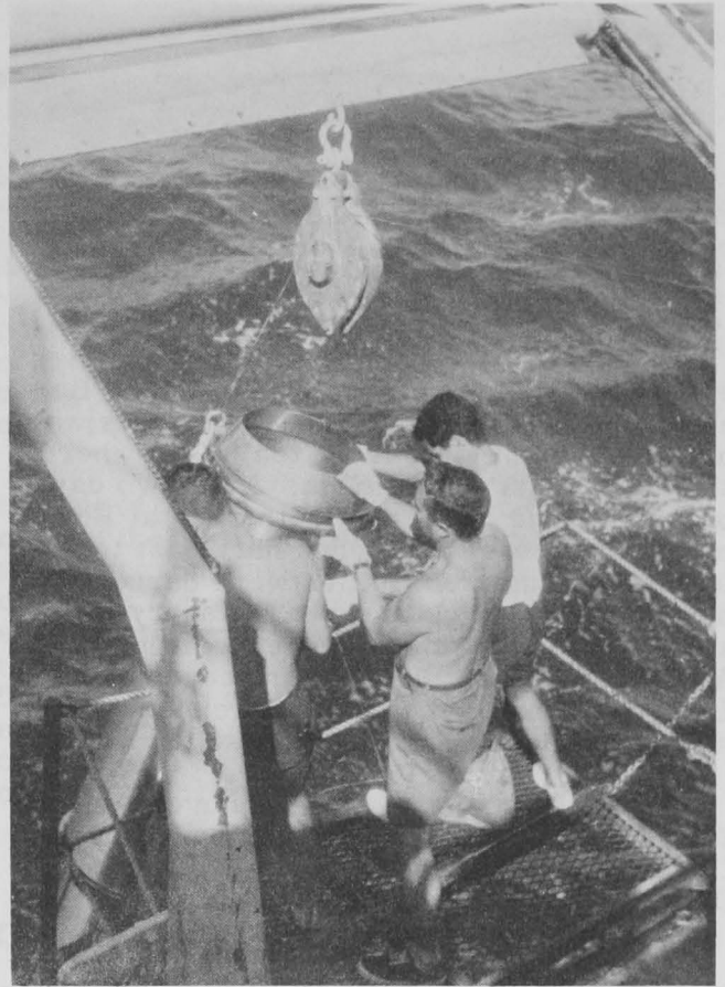
Fig. 3 - Putting over a high-speed plankton sampler which can be towed at 8 knots, thereby capturing fast-swimming organisms that avoid regular plankton nets (which are towed at slower speed).
