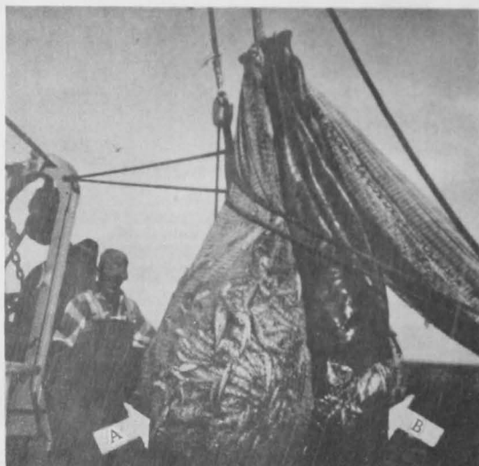
Fig. 1 - 1-inch cover (A) over 2-inch cod-end (B).
