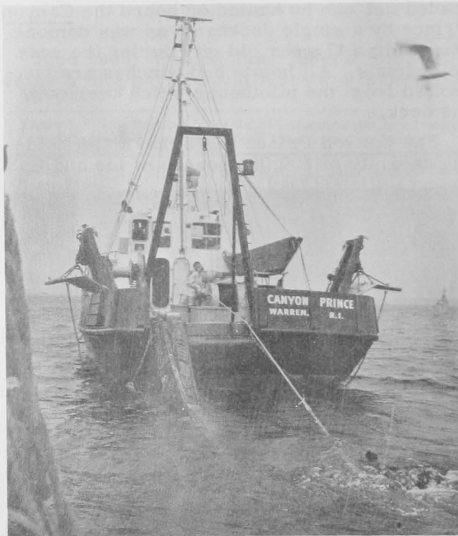
Fig. 3 - Cod-end approaches Canyon Prince ; balance of net to the left is hauled by net drun.
