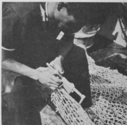
Fig. 2 - Measuring mesh size with mesh gauge.
