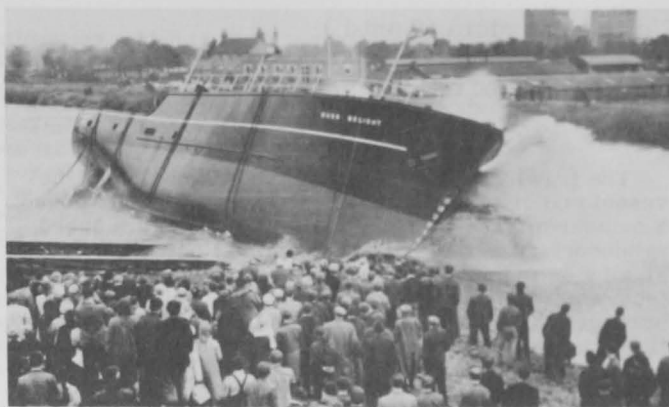
Fig. 2 - Launching of the Ross Delight at Selby, England, shipyard. This is the second of a new class of stern-trawlers termed "push button" trawlers.
