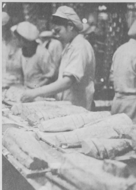
Slicing cooked tuna loins for canning in a cannery located in Hiroshima, Japan.
