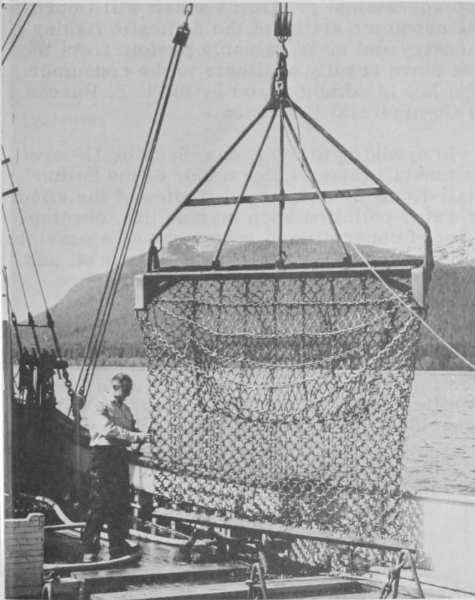
Fig. 2 - Eight-foot scallop dredge used aboard John R. Manning during Cruise 63-1. The inside diameter of the rings is three inches.
