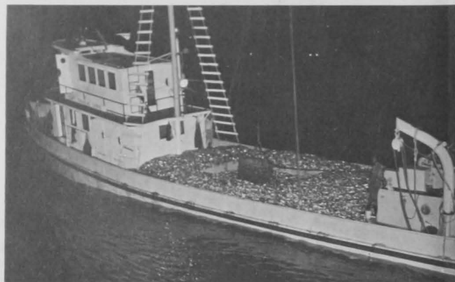
A purse seiner in the Gulf of Mexico with a full load of menhaden.
