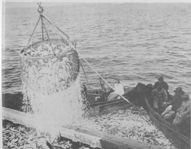
Brailing menhaden from the pocket or bunt of a purse seine. Fish meal, oil, and solubles are produced from menhaden. More modern purse seiners are now equipped with large suction hoses to transfer the fish from the net to the vessel.
