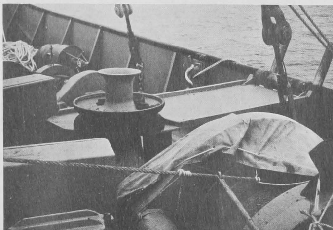
Fig. 2 - Gurdy and rail net roller as adapted on the George B. Kelez .
