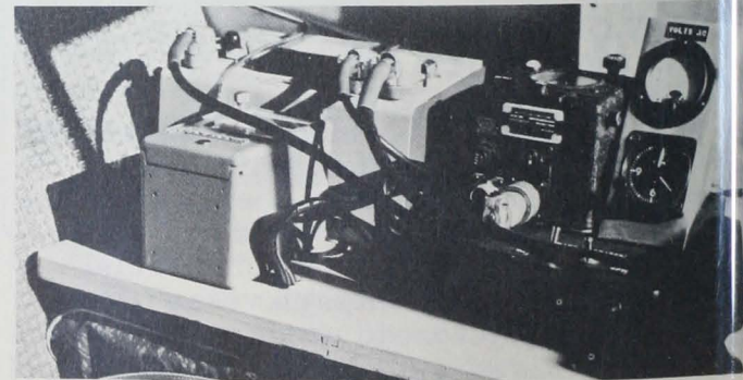
Fig. 2 - Airborne infrared thermometer and accessory equipment positioned in the light aircraft.
