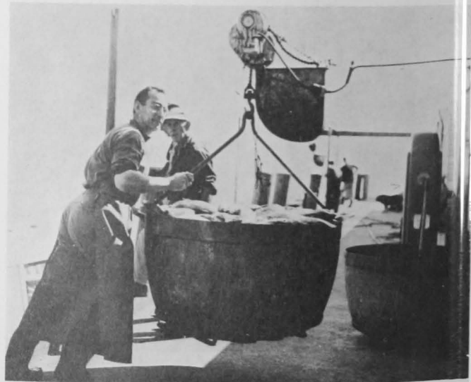
Fig. 12 - The bucket of fish is moved on an overhead trolley into the packing room. The fish are separated by species and packed with ice in wooden boxes for shipment to Boston, New York and other eastern cities.
