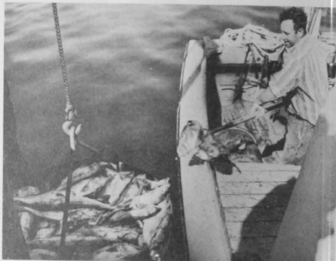
Fig. 11 - A pitch fork is used to transfer the fish from the vessel to the bucket. When the bucket is filled it is hoisted to the deck of the pier.
