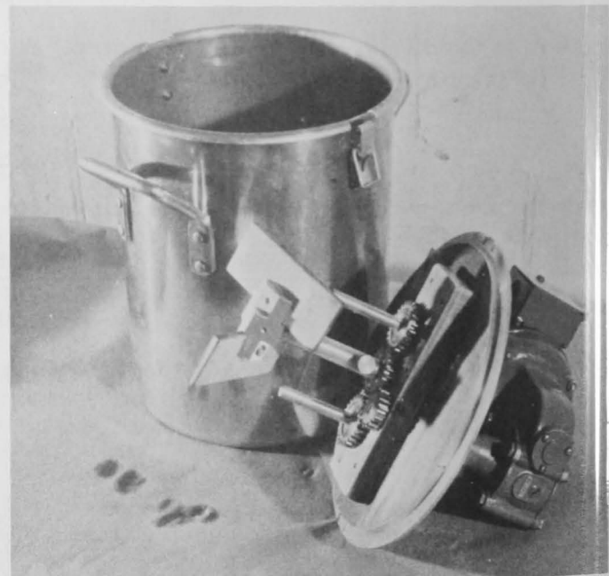
Fig. 1 - This is the debreading machine that is in most general use by shrimp-breeding plants. The geared shafts on each side of the center shaft permit the use of double brushes but these are less effective for removal of breading than the paddle.
