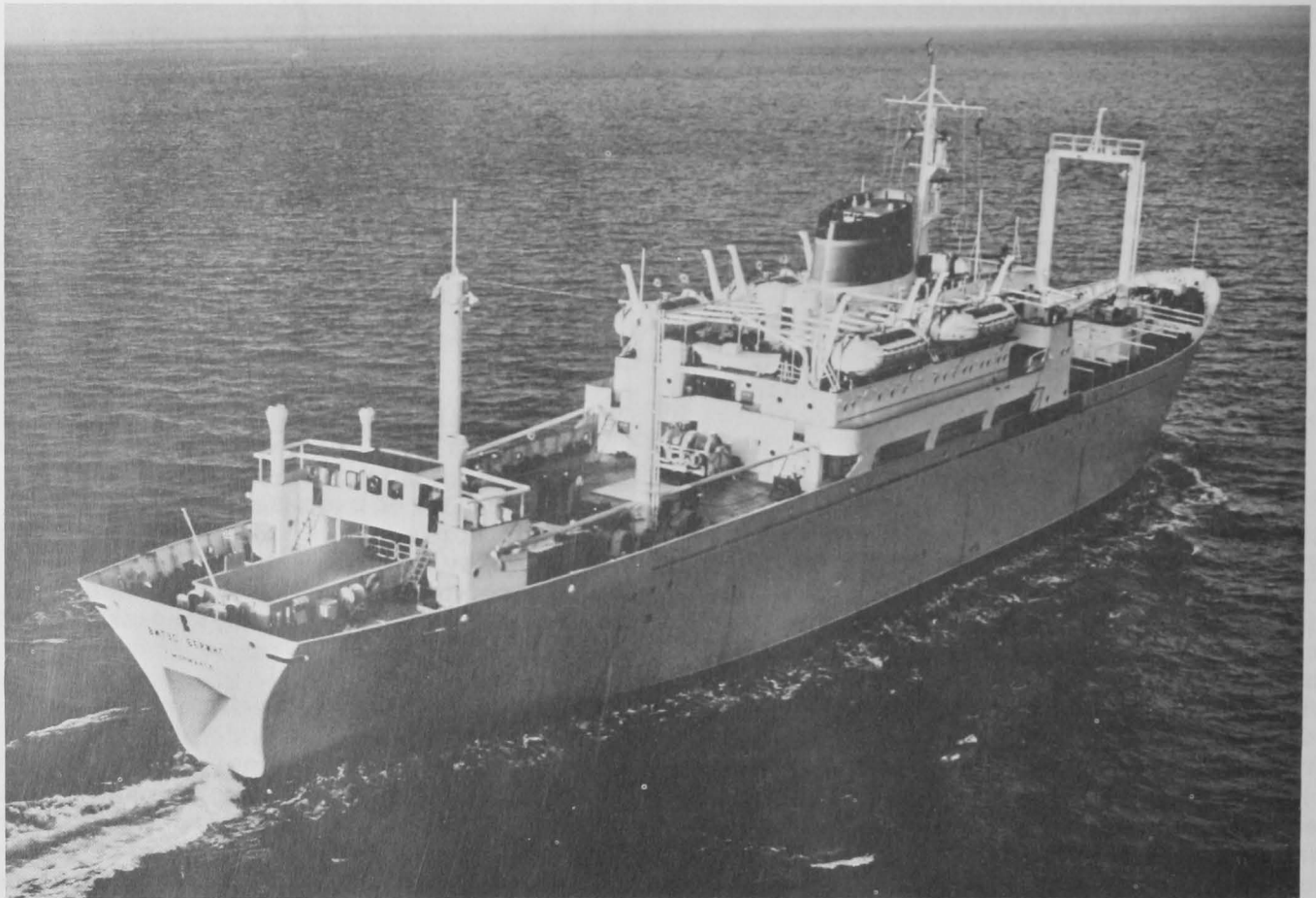
Fig. 1 - Aerial view of the M/S Vitus Bering , fish-freezing vessel built in Denmark for the U.S.S.R. Shows stern ramp for hauling in loaded cod ends and deck layout.
