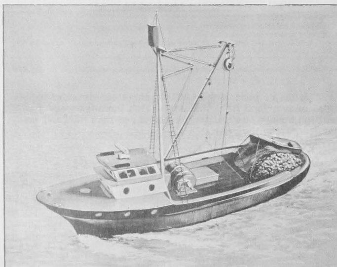
Artist's drawing of the new stern trawler-purse seiner rigged with an automated over-the-stern net-handling system.
