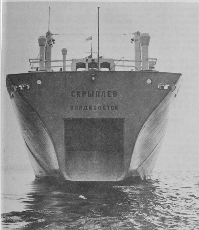
Fig. 2 - Stern view of Soviet fish carrier M/S Skryplev showing stern chute.
