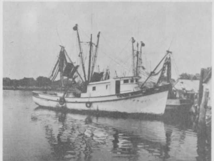
Fig. 3 - Many of the larger trawlers are double-rigged so that they can drag two trawls simultaneously. Note the two pairs of trawl doors hanging from the rigging, one pair on each side of the vessel.
