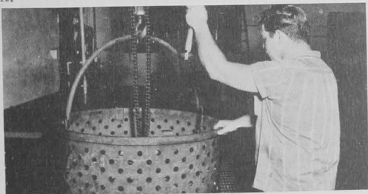
Fig. 40 - The cans of cooked shrimp are immersed in cooling water. Cooling prevents the shrimp from becoming overcooked.
