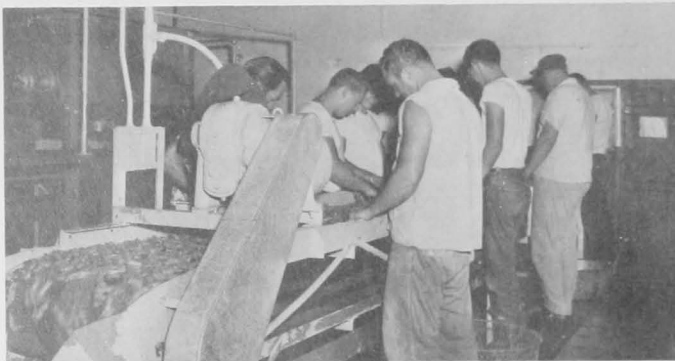
Fig. 6 - The shrimp are passed over an inspection belt, where debris and cull shrimp are removed.
