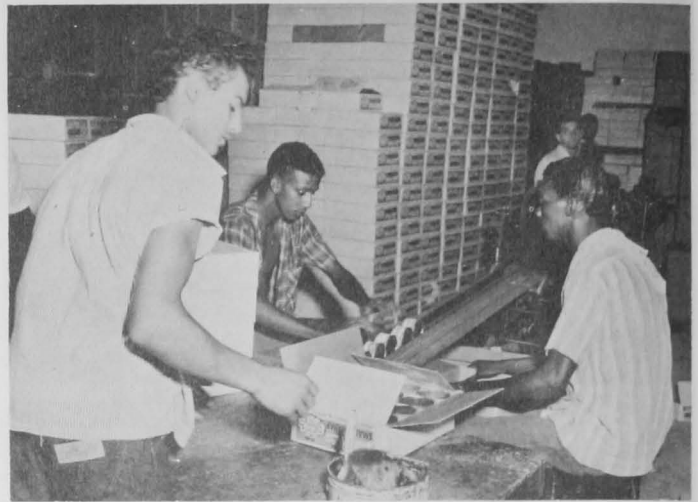
Fig. 43 - After the cans have passed through a labeling machine, they are packed into cartons ready for shipment to the consumer.
