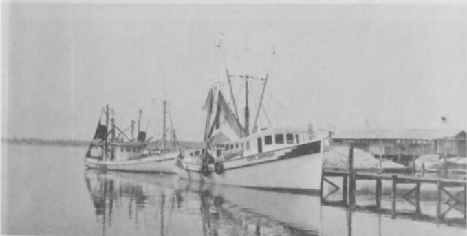
Fig. 2 - Shrimptrawlers vary not only in size but also in design. The vessel in the foreground is a Florida-type trawler with the house well forward. The vessel in back is of the Biloxi type.
