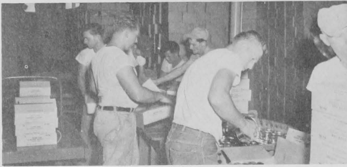
Fig. 42 - The unlabeled cans may be cased for storage, depending on the orders at hand.
