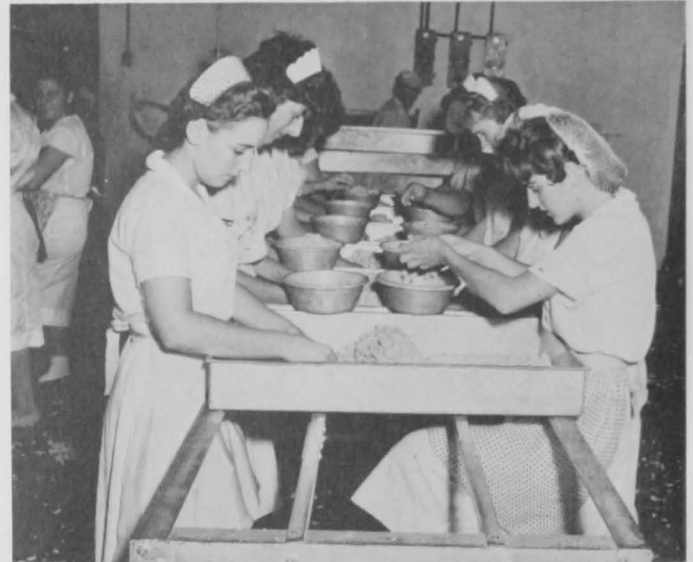
Fig. 31 - Broken shrimp are separated from the perfect ones.
