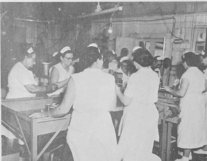
Fig. 32 - The cans are weighed by hand in order to meet the close tolerances required.
