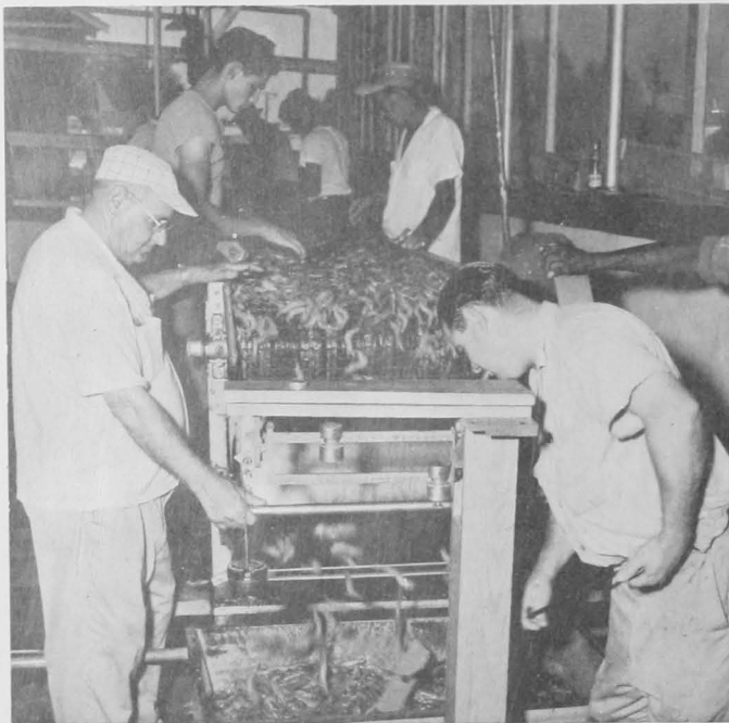
Fig. 8 - The inspected shrimp are conveyed to a weighing basket, which holds 105 pounds or a half barrel of shrimp.
