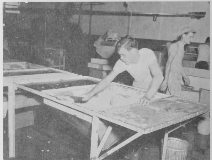
Fig. 45 - The equipment and the plant are thoroughly scrubbed with detergents and chlorine.
