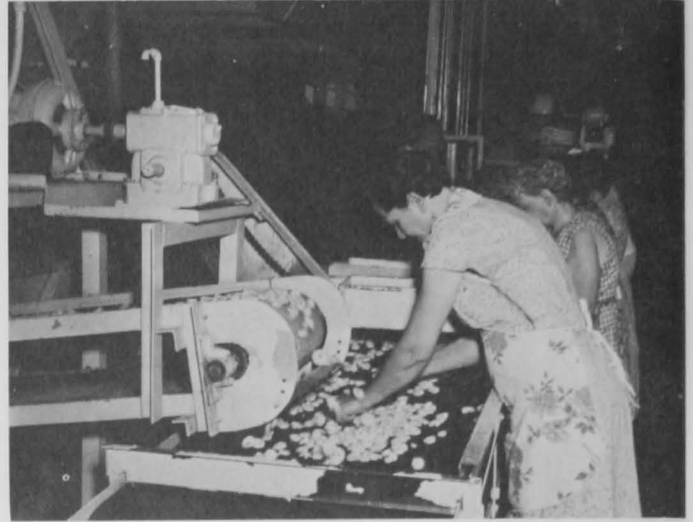
Fig. 29 - When the shrimp have been cooked, they are again inspected. After having passed through the cooker, they develop an attractive pink color and a characteristic curl. This curled shape not only is attractive, but use is made of it later in the mechanical grading of the shrimp for size. Also it is necessary to remove a portion of the moisture in order to get the proper amount in the can for required drained weight cut-out.
