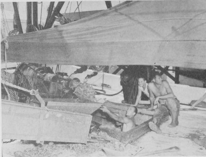
Fig. 4 - Shrimp and ice are shoveled from the hold into a conveyor-hopper. Depending on the location of the plant and on circumstances, shrimp are brought to the plant by either vessel or truck.
