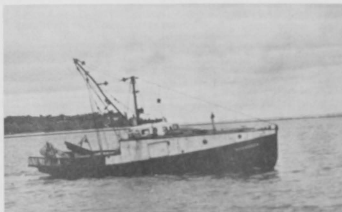
Fig. 3 - M/V Kevinbren , a converted gill-net type vessel used during a part of the explorations.
