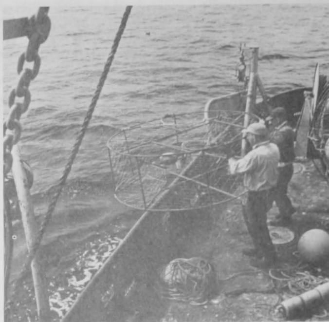
King crab pot being released over the side of the Yaquina on cruise 62-3. The mesh is knit from stainless steel wire. The buoy line used is part polypropylene and part nylon.
