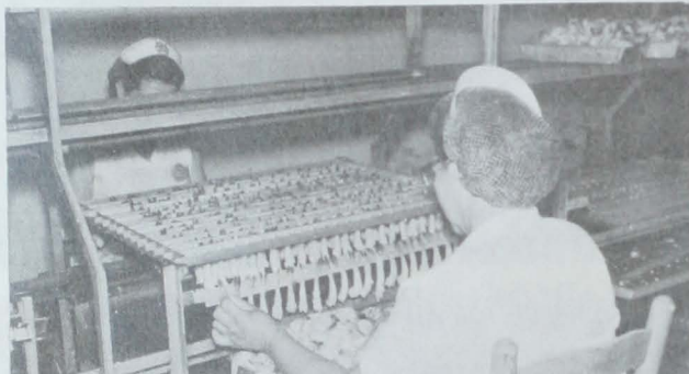
Fig. 27 - One plant has developed a special machine to batter and bread shrimp without breading the fantail. Workers suspend shrimp by the tail from pins on strips.
