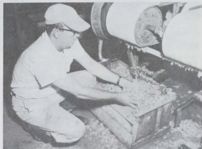
Fig. 19 - The shells discharge from the conveyor belts under the work table. Weight lost in peeling is from 15 to 25 percent.
