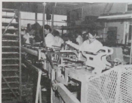
Fig. 43 - A typical wrapping machine. Rack at left is being filled with wrapped boxes. It then will be rolled into a blast freezer.
