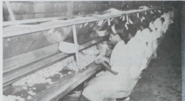
Fig. 13 - After being graded, the shrimp are peeled and deveined. For the best grade of product, this operation is still carried out by hand. Bins feed the shell-on shrimp to the workers.
