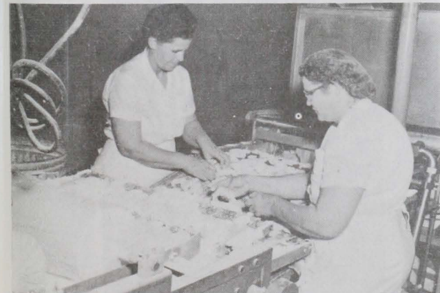
Fig. 35 - Some redistributing is needed before the shrimp go under the second batter curtain. Note the plastic covers on the rolls. Direction of motion is to the right.
