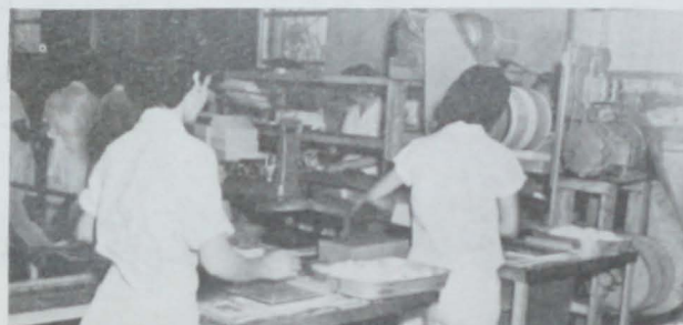
Fig. 41 - These workers are checking weight of institutional size (5-pound) packages. Conveyor at far left carries the packages to the wrapping machine.
