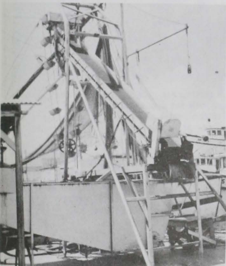
Fig. 6 - Conveyor in withdrawn position. Shrimp mixed with ice drop into the tank in center left.
