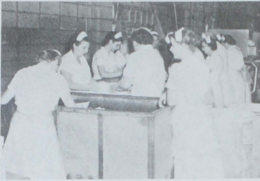
Fig. 22 - In some operations the peeled and deveined shrimp are predusted by hand before going to the breading machine. Many plants use two machines in tandem, eliminating the predusting operation.
