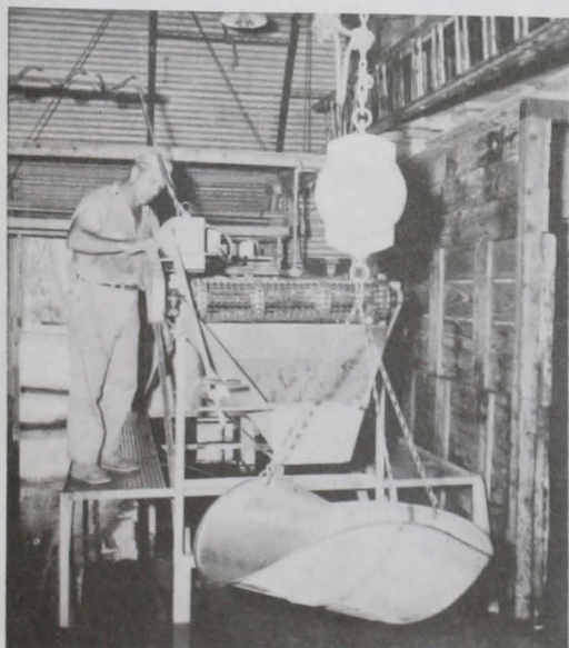
Fig. 8 - The conveyor from the wash tank discharges the shrimp directly to a large scale-scoop. In each "100-pound box," 105 pounds are packed to allow for water and ice. These plants handle only fresh shrimp, which are destined for either the breeding plant or the freezer.
