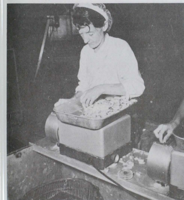
Fig. 18 - This machine, a deveiner, slits the shell and shrimp so the sand vein can be washed out, but the shell must be removed by hand.
