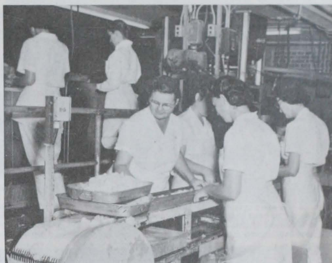
Fig. 17 - The machine-peeled shrimp must be inspected for adhering pieces of shell and "sand veins," which would lower the grade of the frozen breaded product. Two machine peelers are visible in the background.
