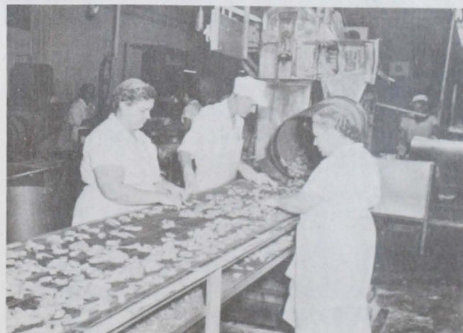
Fig. 21 - When only one breading machine is used, the shrimp may be predestered by tumbling shrimp and dry batter-mix in a revolving drum. Workers distribute predestered shrimp on the wire belt of the breader.
