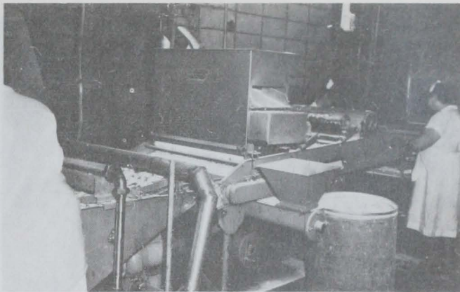
Fig. 32 - After the batter spray, a blast of air from the duct shown in left center blows off excess batter. This operation reduces excessive pickup and loss of breading.
