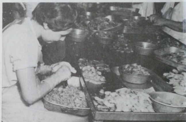
Fig. 15 - Tables and pans used by the hand peelers are either stainless steel or aluminum to facilitate cleaning and sterilization. The plant is washed down thoroughly after each shift.
