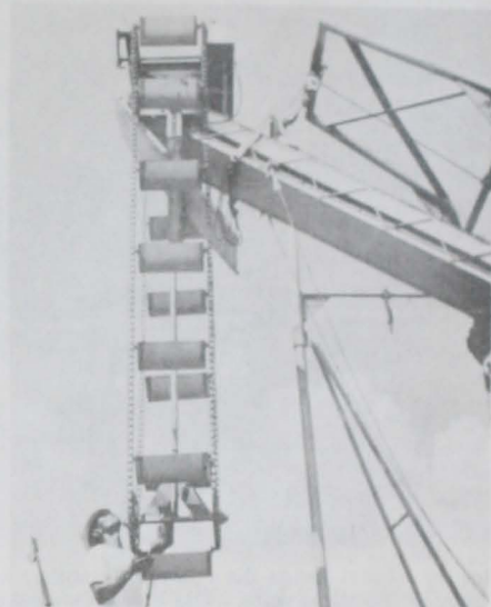
Fig. 5 - The bucket leg can be lowered into the boat hold. Note pulley on the upper right.
