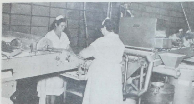
Fig. 37 - The end of the first breeder, the second batter unit and second breeder, and in the background, the first of the packers can all be seen in normal sequence.
