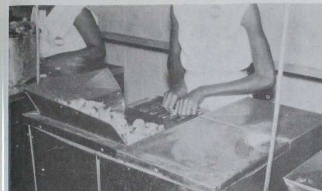
Fig. 16 - Machines have been developed to speed peeling and deveining. An operator positions the shrimp as she feeds them one by one into the machine.
