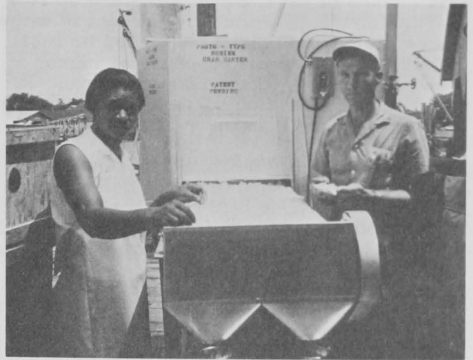
Fig. 2 - Francis Altman, right, beside the crab-picking machine he invented. At Oriental, N. C., a crab-processing plant employee feeds bobbed crabs into the machine where the meat is separated from the shell. The machine is patented.
