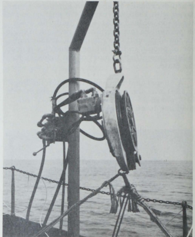
Hydraulic crab and long-line block used to retrieve fishing gear.
