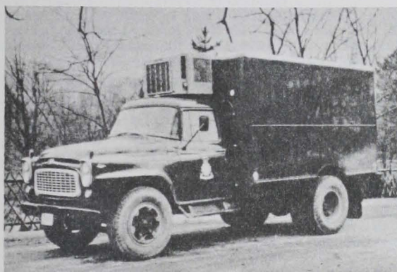
New refrigerated truck, which will operate out of Port aux Choix, will service bait holding units on the northwest coast of Newfoundland. Truck has a maximum load capacity of 14,700 pounds of bait.
