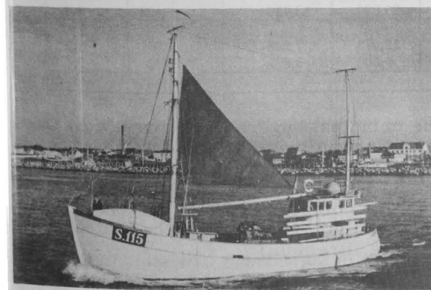
A typical Danish fishing vessel. This vessel, built in 1960, is 52.3 gross tons, has a 248 hp. motor and its home port is Skagen.
