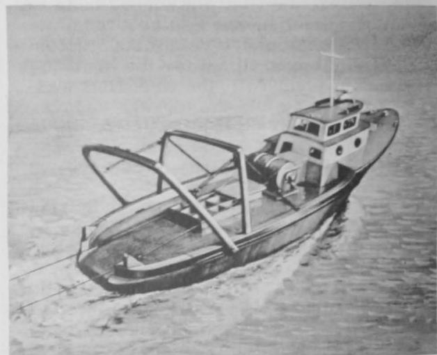
Fig. 1 - New 76-foot semiautomated stern trawler-purse seiner rigged for stern trawling.
