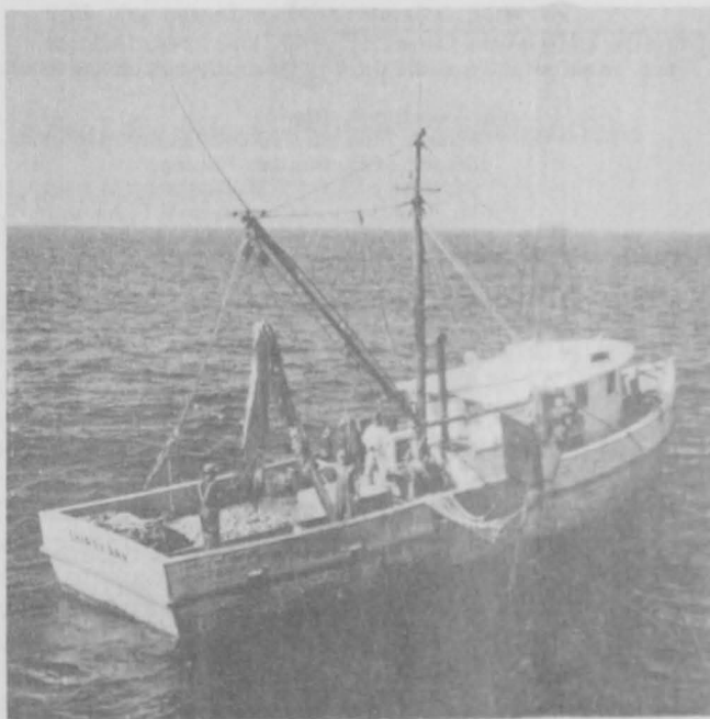
Fig. 7 - A single-rigged scallop trawler on the grounds. The trawl is dragged from the starboard outrigger boom.
