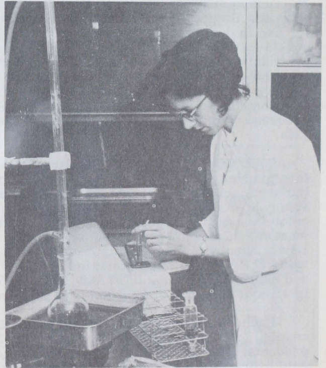
Fig. 1 - Chemist analyzing smoked mullet fillets for rancidity by the thiobarbituric acid method.
