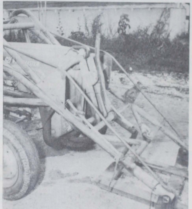
Fig. 8 - The lever (center) that positions the platform during the lift has a unique shape. This lever slides over the "nose" on the forward edge of the mounting frame.
