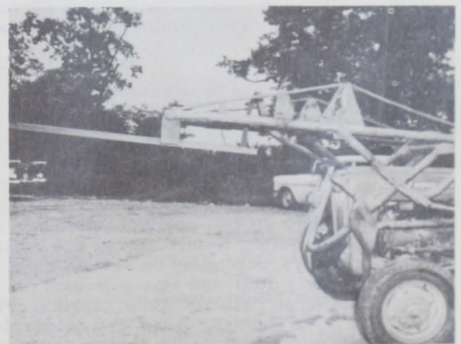
Fig. 9 - Shown from another angle is the relative position of the framework when the fork is raised.
