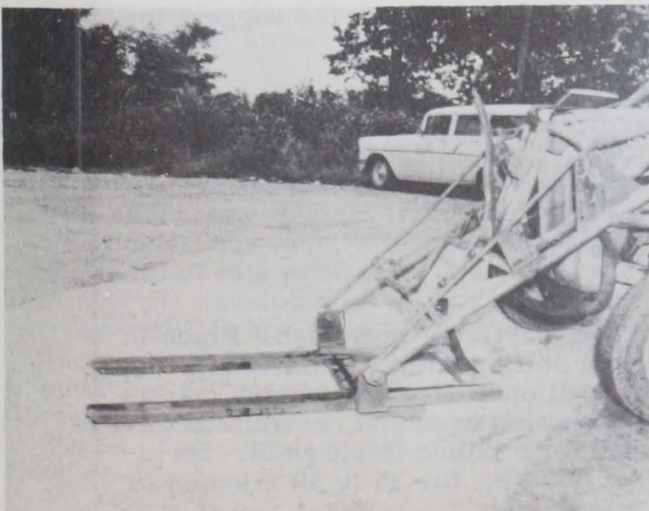
Fig. 7 - The fork lies perfectly flat at floor level.
