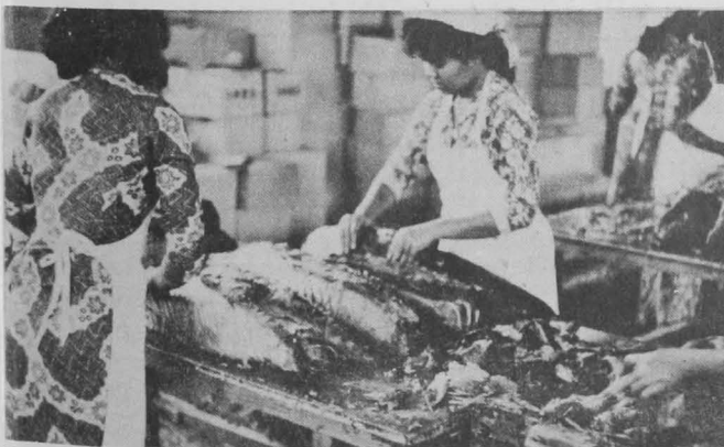
Fig. 10 - After cooling, the bones, dark meat, and skin are removed from the cooked tuna.
