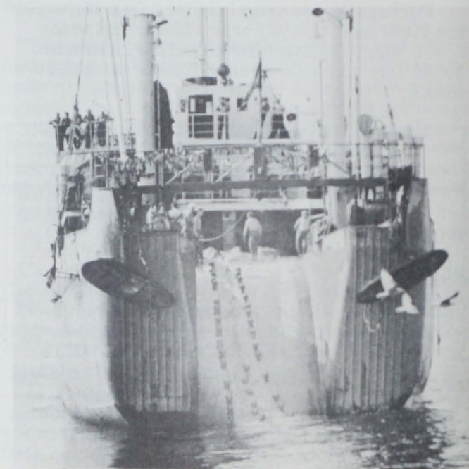
Russian "Maiakovski"-type stern trawler fishing on the "Northern Edge" of Georges Bank in October 1961. Leading portion of cod end being hauled up the stern ramp of the trawler.
