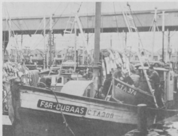
Fig. 8 - A spiny lobster vessel with a few crew members relaxing around one of the dinghies used to tend the lobster pots. The pots, with their buoy lines and the strings of cork floats that form the buoys, are draped over the boom.
