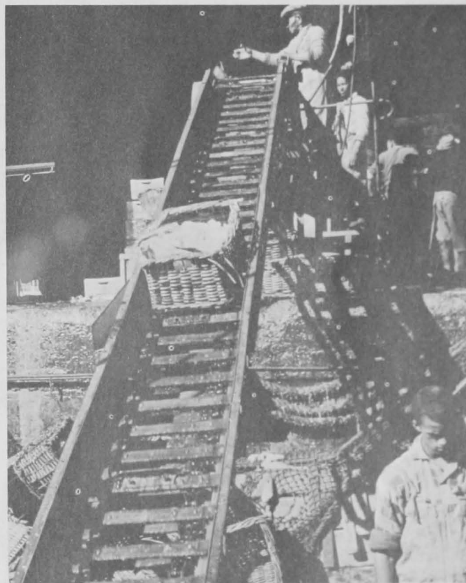
Fig. 3 - The filled baskets of stockfish and other species caught by the trawlers are placed on a mechanical conveyor that raises them to the pier where the fish are sorted and boxed.
