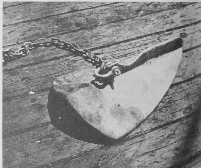
Fig. 3 - Depressor used on each of the wing ends of midwater trawl. Depressors are cast of bronze and weigh approximately 45 pounds each.
