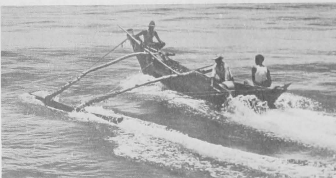
Fig. 3 - Speed trials of a small outrigger canoe fitted with a 10-hp. outboard motor on the south coast of Ceylon. FAO expert aided in introducing outboard motors for use on this type of boat.
